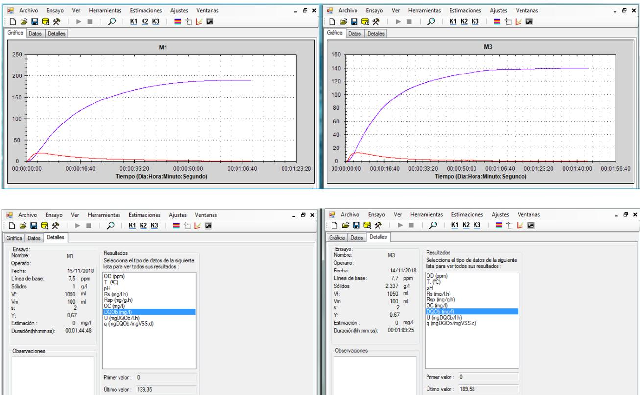
Simultaneous respirograms and results from, the tests performed in each reactor
