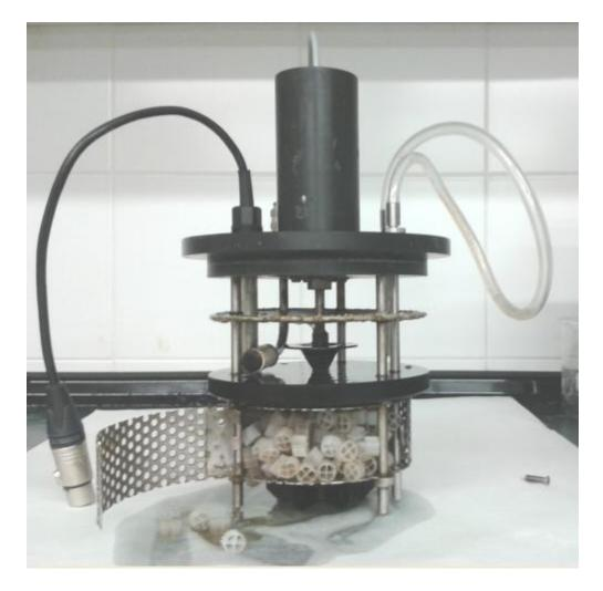
2. Place the filled cage into de reactor vessel which is loaded with the surrounding mixed-liquor of the actual process
