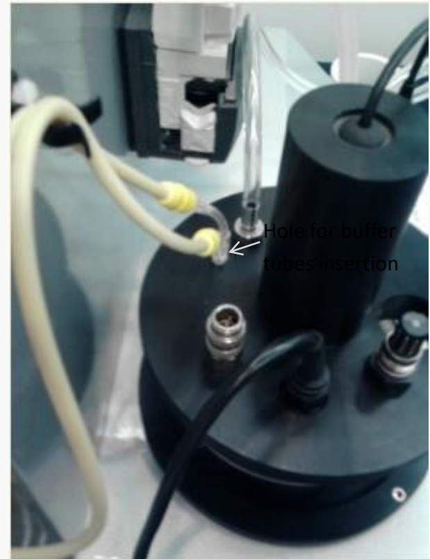
Automatic pH buffers dosage in the reactor
