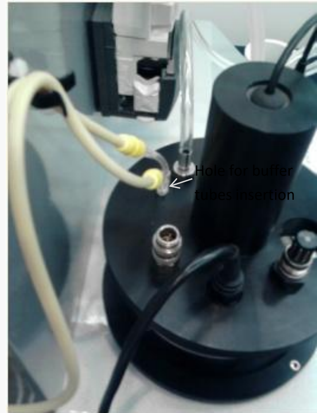
Automatic pH buffers dosage in the reactor
