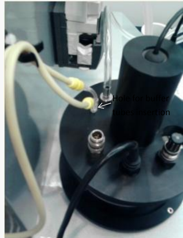
Automatic pH buffers dosage in the reactor
