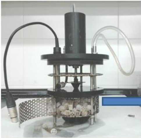
Biomass-carriers loading in the reactor-cage
