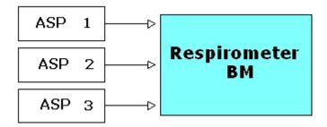
One common application for that type of working mode is to take the pulse to each of the mixed-liquors samples coming from the treatment plants. On that way we can make an screening of the samples with potential problems and then go more in deep, with other respirometry analysis.
