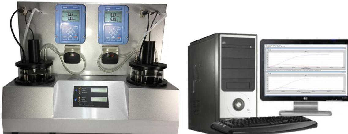
*The two reactors system saves time, by allowing two tests to run simultaneously on identical or different conditions of pH, Temperature, Oxygen and sample volumes*
