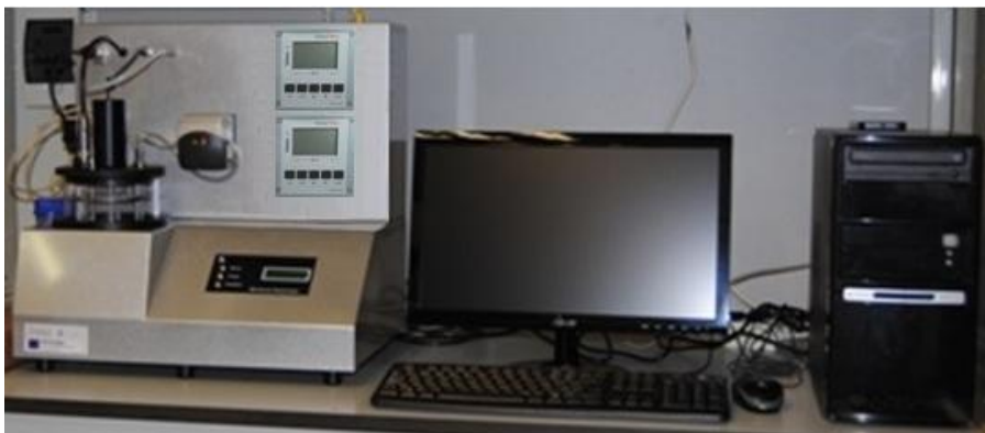
Figure 1. BM-Advance respirometry system
