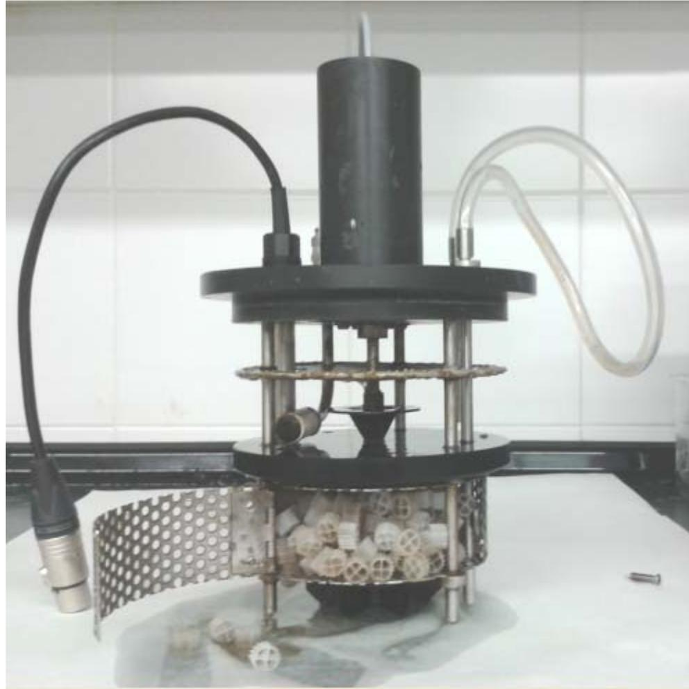
2. Place the filled cage into de reactor vessel loaded with surrounding mixed-liquor of the actual process
